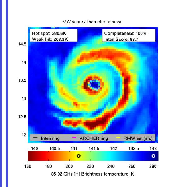
The ARCHER algorithm uses passive microwave imagery in the 85-92 GHz range to objectively estimate eye size and TC organizational/structure characteristics. Eyewall characteristics (intensity and completeness) are used by SATCON to determine any needed eye size corrections. ARCHER scores are used in the motion component logic of SATCON, and are also part of the SSMIS MSW algorithm. ARCHER is currently an integral component of the ADT v8.1.4.
